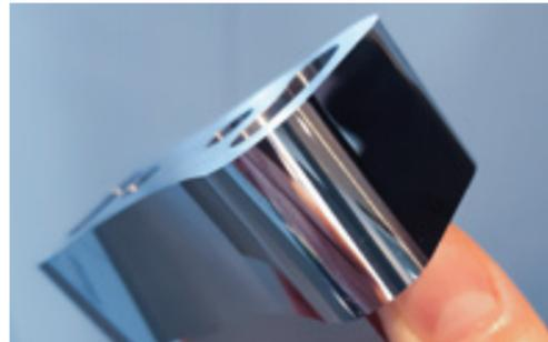
Milling, hard milling and coordinate/contour grinding processes are perfectly combined on one machine. It is possible to decide on the optimum machining strategy on a case-by-case basis and in a highly flexible manner, based on the specific requirements of a workpiece. As a result of complete machining in a single setup, an enormous reduction in throughput times, high-precision finishing and, at the same time, greater process reliability can be achieved.
