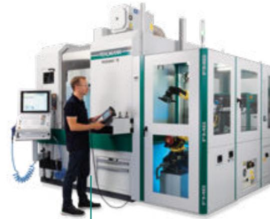
Modular 6-axis robot system for blank parts handling
