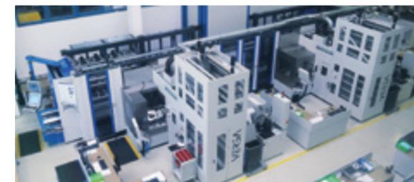
Linear automation solution consisting of two VERSA 825 with rack magazines for up to 346 tools each
