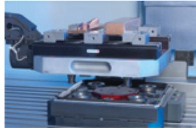
The workpiece feeding system with pallet handling is perfectly suited for medium-sized batches and single parts. Various clamping devices may be mounted on the pallets without having to program a robot.
