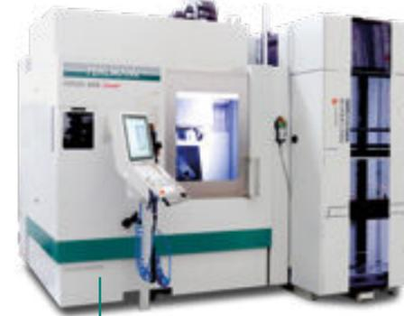
Erowa Robot Compact workpiece loading system for pallets
