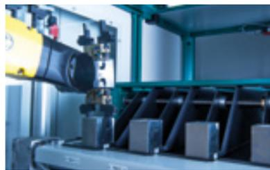
Robotic parts handling with compact and modular 6-axis robot system for all-around processing of round as well as angular blanks.
