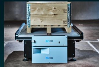
*ROEQ GuardCom enables safe, effective and reliable transfer of goods between AMRs and conveyor stations via coded light sensors that provide seamless communication between the equipment.*
